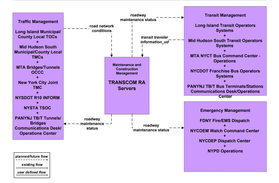
MC07 - Roadway Maintenance and Construction TRANSCOM
